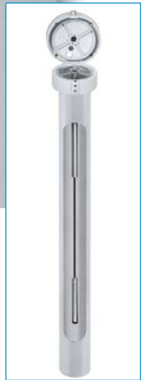
OTT ITC with Orpheus Mini Pressure/Temperature Logger deployed in a 4-inch well.
